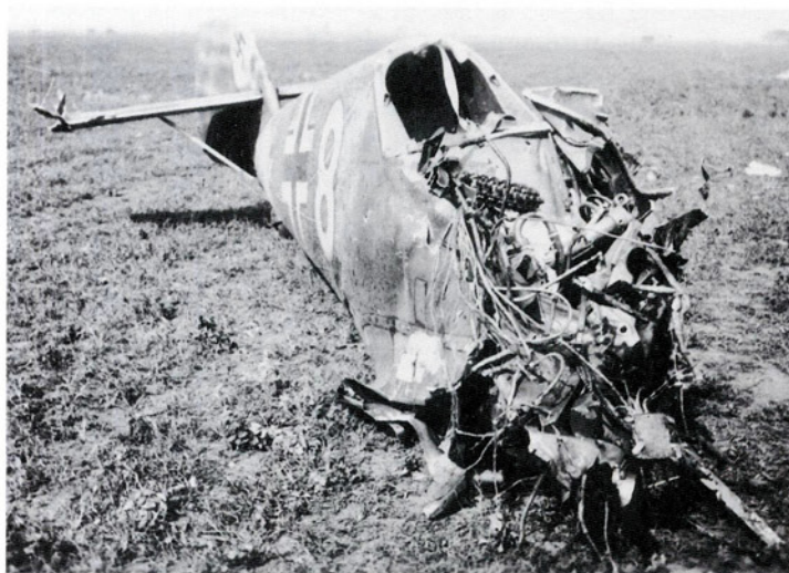
ABOVE AND ABOVE RIGHT: Two views of 'White 8' of 1.(J)/LG 2 which was destroyed at Zilistea in Rumania. Unfortunately date and exact circumstance are not known although the condition of the wreckage suggests a landing accident.
