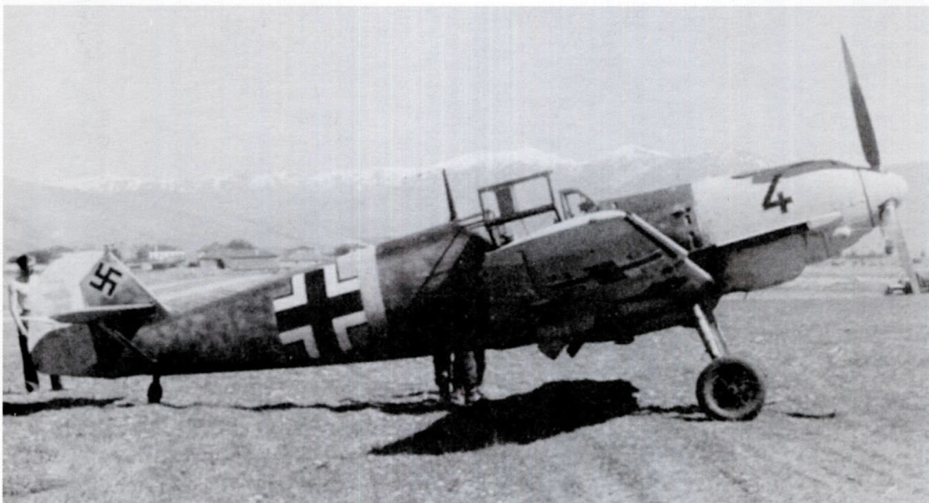
RIGHT: The instruction regarding the application of the yellow fuselage bands which were applied to most aircraft during the Balkans campaign seems to have been fairly liberally interpreted, resulting in a number of variations in band width and location. On this Bf 109 E-7, 'Black 4' of III./JG 27, the band has been applied in such a way that it borders the forward edge of the fuselage Balkenkreuz.
